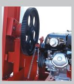
Double V-belt/gear drive. Allows larger, heavier mixes. Cast-steel pulleys increase durability. Idler wheel provides easy, positive engagement.
