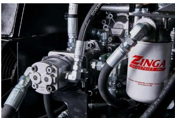
**100% hydraulic drive.** No V belts, pulleys, clutches or mechanical gear reductions.
