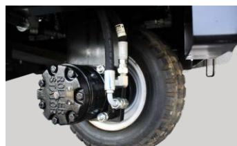
The All-Wheel Drive Buggy is equipped with a powerful steering drive motor for optimum performance. A single over-sized tire provides superior traction.
