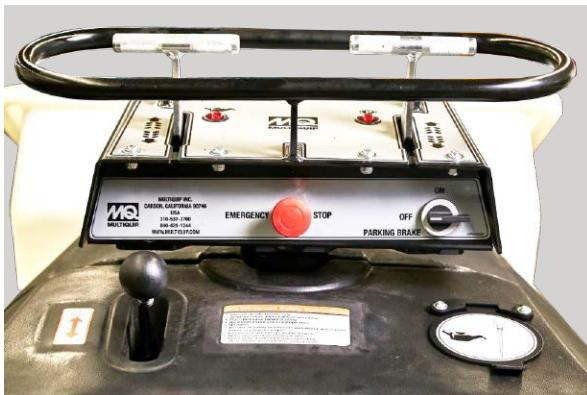
**Dual control handles** provide consistent tracking, easy steering, and minimized operator fatigue. (WTB-16 shown)
