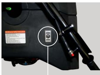
Toggle switch allows operator to easily switch from two-wheel drive to all-wheel drive.
