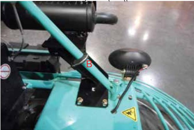
**Figure 9. Muffler Vibration Clamp Installation**
