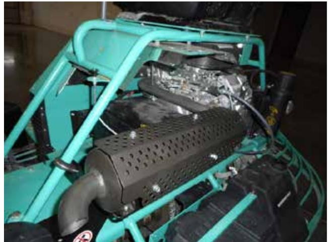
**Figure 11. New Muffler Installed**
