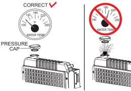
Figure 45. Radiator Pressure Cap Removal
