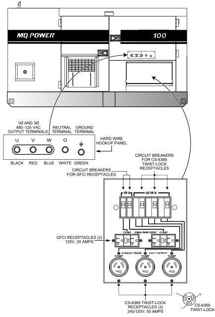
Figure 9. Output Terminal Panel
