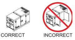
Figure 30. Engine Enclosure Doors
