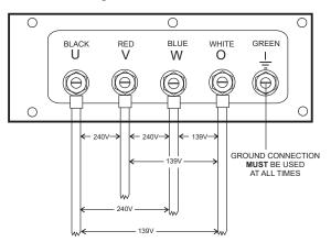
Figure 18. UVWO Terminal Lugs (3-Phase 240-Volt Connections)
