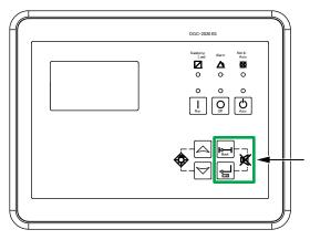
Figure 55. Digital Controller (Alarm Silence Button)
