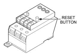
Figure 14. Overcurrent Relay
