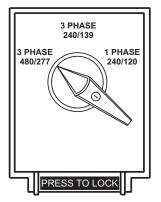
Figure 21. Voltage Selector Switch (3-Phase 480/277-Volt Position)
