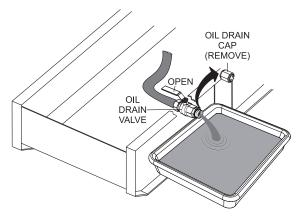
Figure 43. Draining Engine Oil
