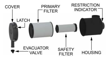
Figure 41. Engine Air Cleaner Components
