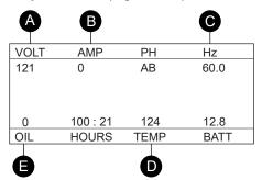
Figure 34. Controller Display
