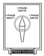
Figure 17. Voltage Selector Switch (3-Phase 240/139-Volt Position)
