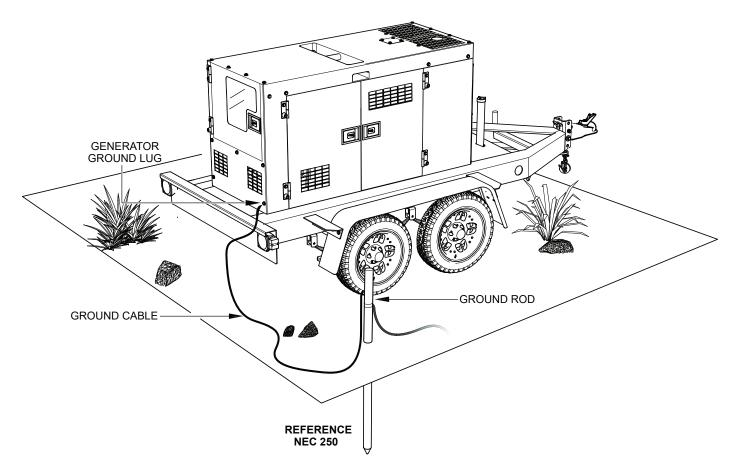
Figure 3. Typical Generator Grounding Application
