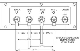
Figure 22. UVWO Terminal Lugs (3-Phase 480-Volt Connections)
