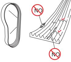
Figure 48. Drive Belt Inspection
