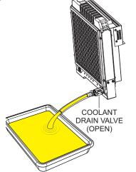
Figure 46. Draining Engine Coolant
