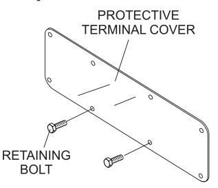
Figure 12. Protective Terminal Cover (Output Terminal Lugs)
