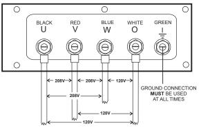
Figure 20. UVWO Terminal Lugs (3-Phase 208-Volt / 1-Phase 120-Volt Connections)
