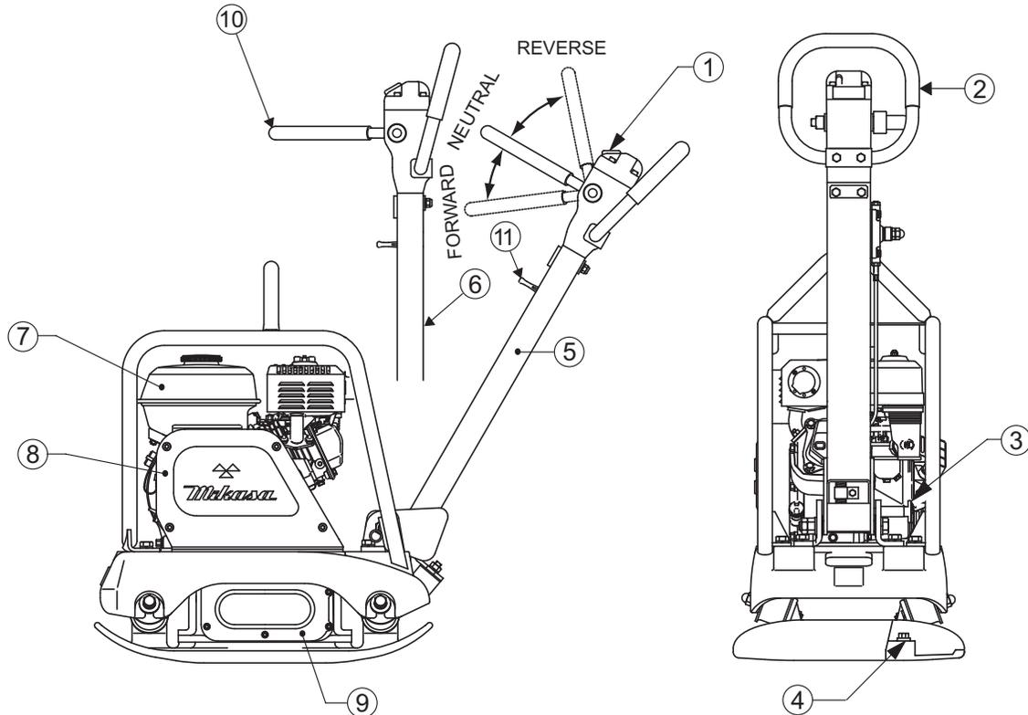
**Figure 2. Compactor Components**
