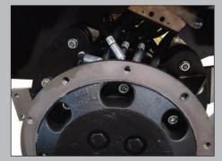
**Hydraulic Hose Network** Easily accessed through the drums with no special tools required. All hoses are routed to prevent wear and numbered for easy identification.
