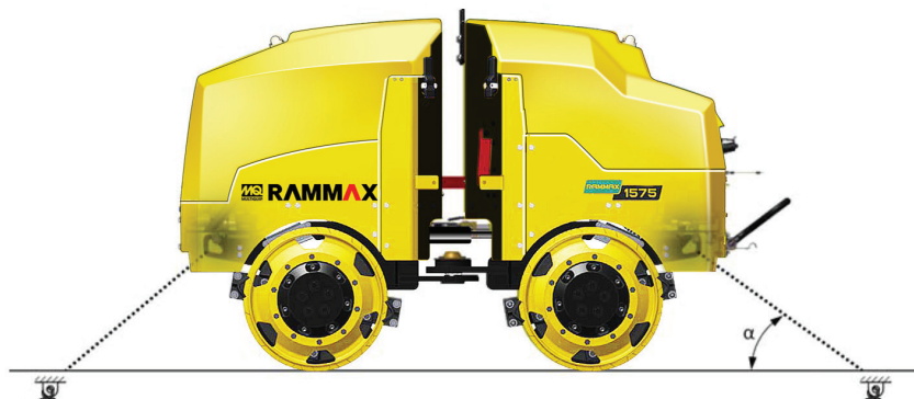
Fig. 12-3 Lashing the roller/side view
