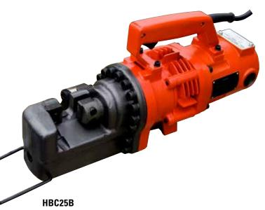
Maximum Cutting Diameter In (mm) 1 (25) #8 rebar grade 60 Voltage/Amperage 115V 60Hz 13 amps
