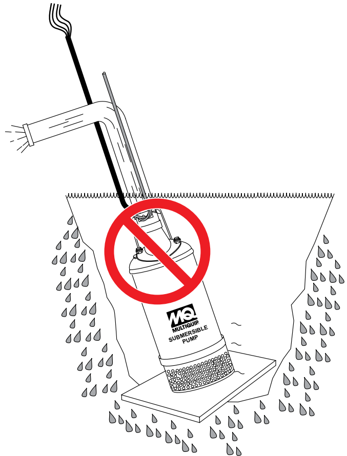
Figure 21. Submersible Pump Upright Position (Incorrect)
