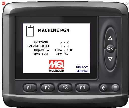
Figure 5. Hydraulic Oil Level Display
