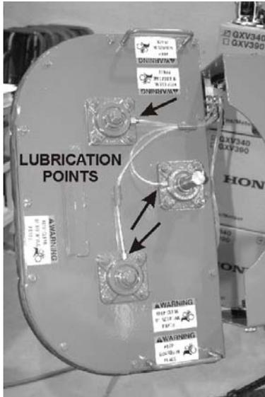
Figure 51. Lubrication Points
