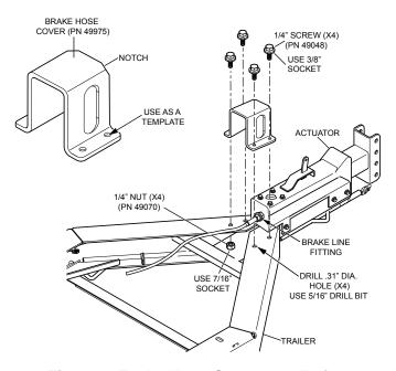
Figure 2. Brake Hose Cover Installation
