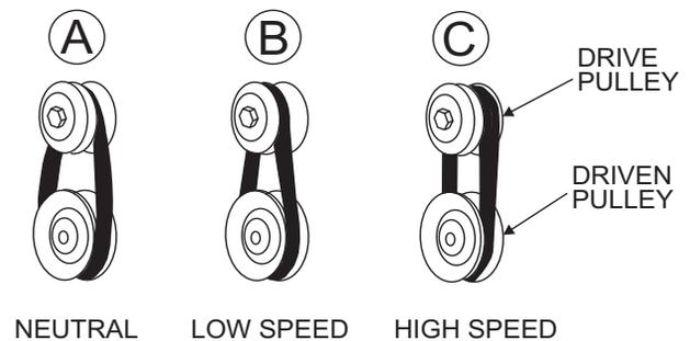
Figure 25. Pulley Conditions
