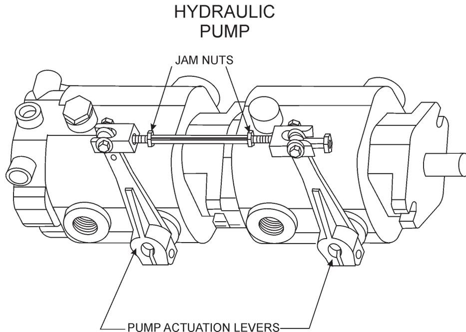
**Figure 17. Pump Actuation Levers/Speed Control Rod**
