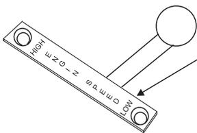
WHEN STARTING ENGINE, PLACE THROTTLE CONTROL LEVER IN LOW POSITION
