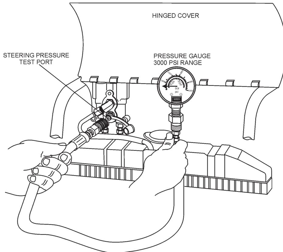
Figure 20. Pressure Gauge (Left Steering Valve)
