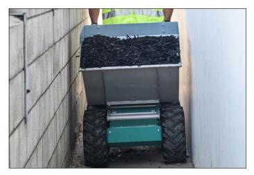
**Optional 2.8 ft<sup>3</sup> steel clip-on tub** — **TT7** — allows access through narrow 32-inch passageways.
