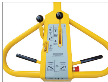
Multi-functional handle controls forward and reverse travel, water flow to the drum, vibration and the emergency stop feature.
