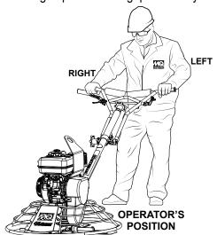
Figure 1. Operator's Position
