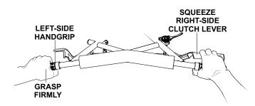
Figure 3. Engaging The Clutch
