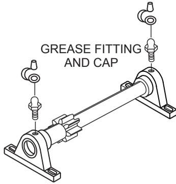
**Figure 34. Grease Fittings (Countershaft)**
