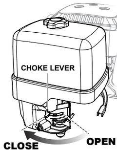
Figure 15. Choke Lever
