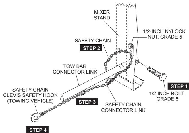
Figure 1. Tow Bar and Safety Chain Installation
