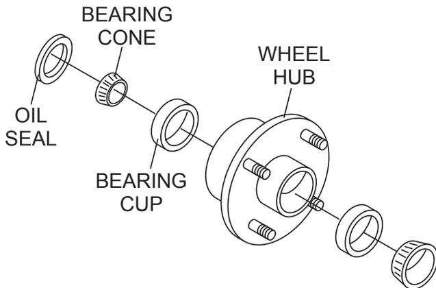
**Figure 35. Wheel Hub and Bearings**
