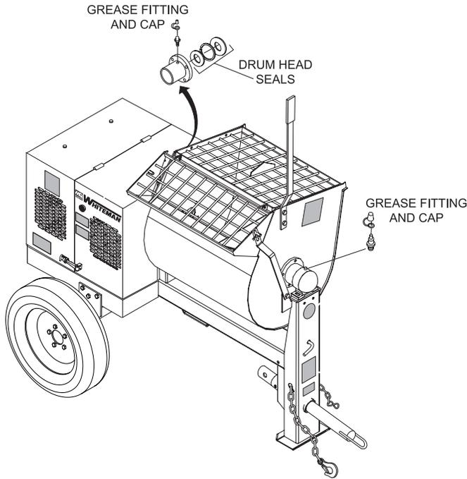
Figure 32. Grease Fittings (Drum Head Seals)
