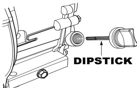
**Figure 7. Engine Oil Dipstick (Removal)**
