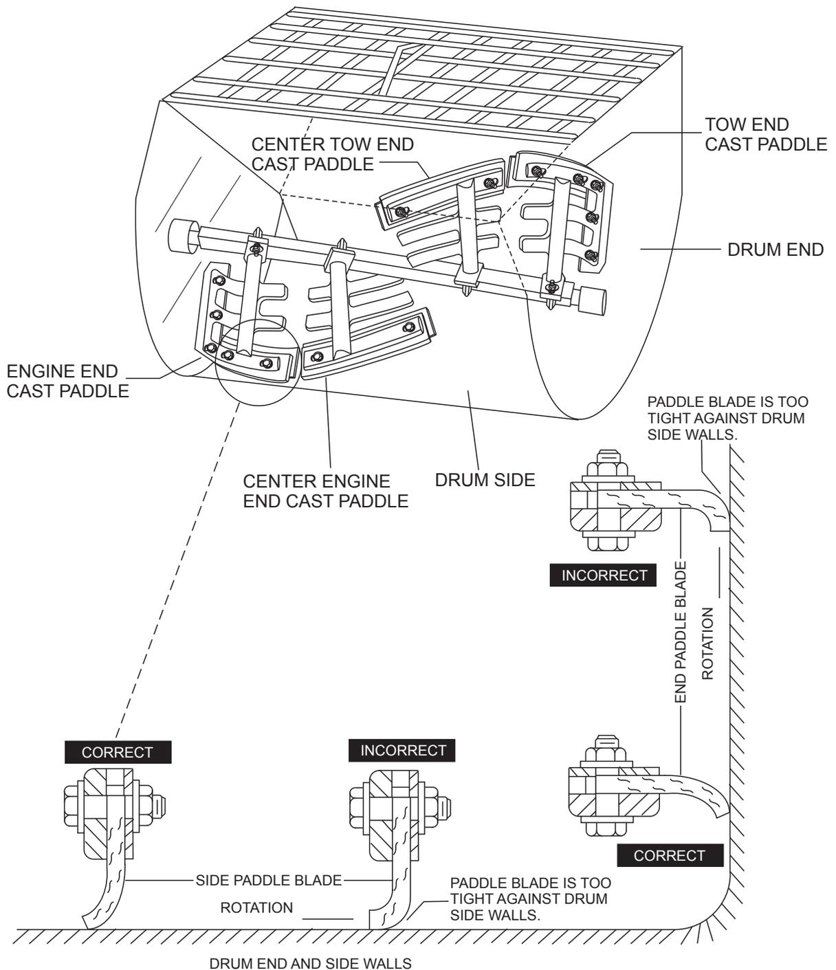
**Figure 13. Paddle Blade Adjustment**
