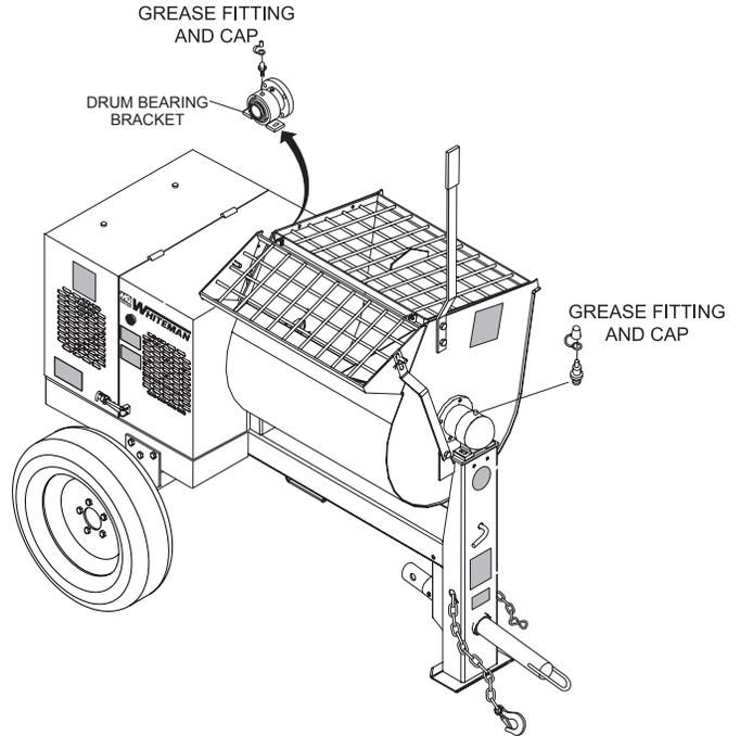
Figure 33. Grease Fittings (Dumping Mechanism)
