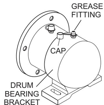
Figure 12. Grease Fittings Drum Bearing Bracket
