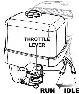
Figure 16. Throttle Lever
