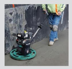
Allows finishing within 7/16" of any obstruction
